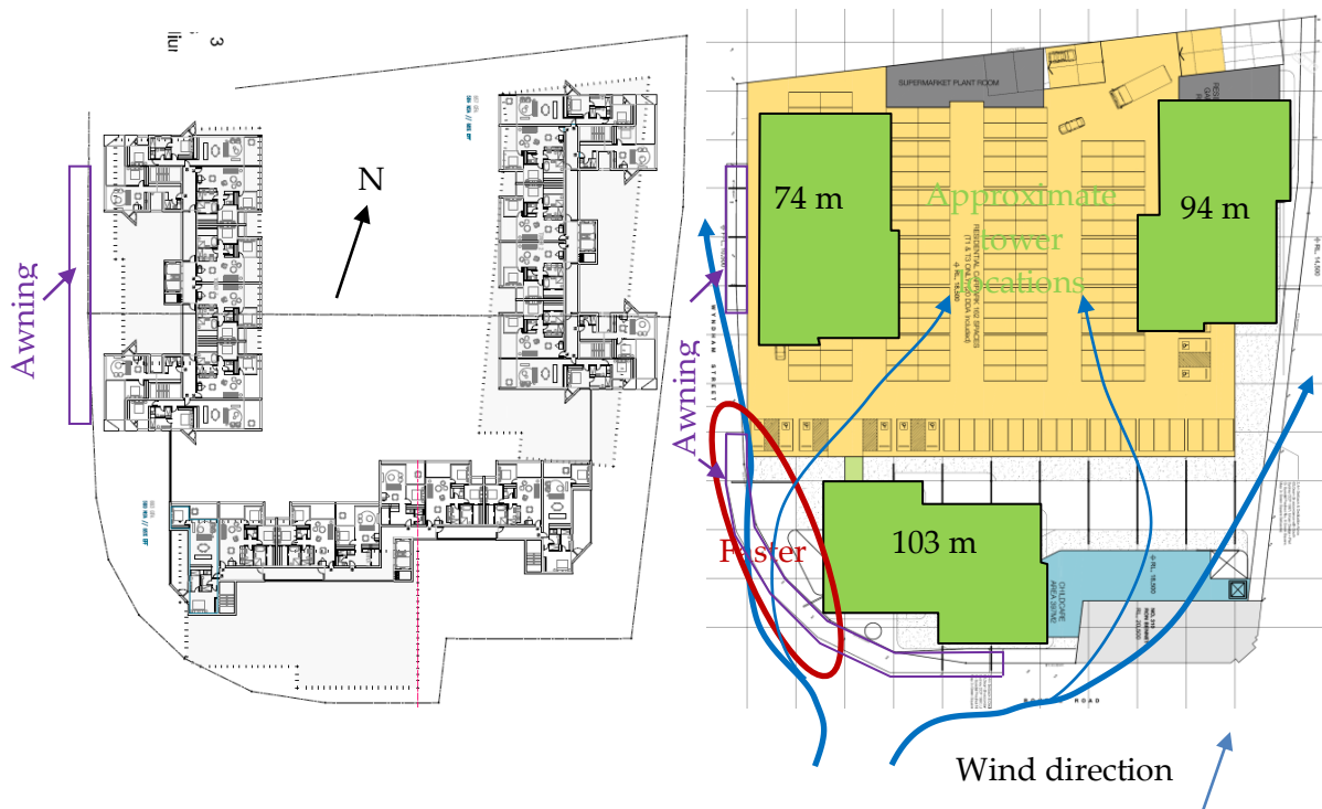
Figure 1: Plan view of the proposed development: revised (L), and previous scheme of April 2015 showing wind flow patterns for winds from the south (R)
